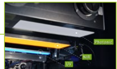
In-line Post-treatment Processes: Drying and/or Curing Modules (UV, NIR, Photonic, etc.)
